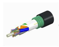
Fiber OSP cable, LazrSPEED® Single Jacket/Single Armor, 96 fiber, Gel-Free, Stranded Loose Tube, Multimode OM4, Feet jacket marking, Black jacket color
