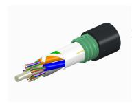
Fiber OSP cable, LazrSPEED® Single Jacket/Single Armor, Gel-Free, Stranded Loose Tube, 24 fibers, Multimode OM4, Feet jacket marking, Black jacket color
