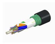
Fiber OSP cable, LazrSPEED® Single Jacket/Single Armor, Gel-Free, Stranded Loose Tube, 12 fibers, Multimode OM4, Feet jacket marking, Black jacket color
