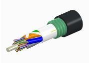
Fiber OSP cable, LazrSPEED® Single Jacket/Single Armor, , 60 fibersGel-Free, Stranded Loose Tube, Multimode OM3, Feet jacket marking, Black jacket color
