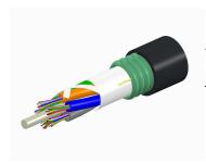
Fiber OSP cable, LazrSPEED® Single Jacket/Single Armor, Gel-Free, 36 fibers, Stranded Loose Tube, Multimode OM3, Feet jacket marking, Black jacket color
