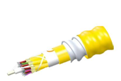
Distribution cables are color coded 900um tight buffered fibers for easy connectorization. Fiber counts above 24 are unitized for manageability. All fiber types are bend insensitive. Singlemode fiber is ITU-T G.657.A1 compliant as well as backwards compatible to G.652.D
