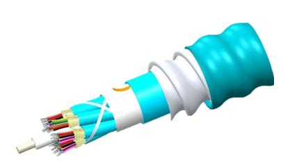
Distribution cables are color coded 900um tight buffered fibers for easy connectorization. Fiber counts above 24 are unitized for manageability. All fiber types are bend insensitive. Singlemode fiber is ITU-T G.657.A1 compliant as well as backwards compatible to G.652.D
