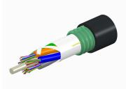
Fiber OSP cable, LazrSPEED® Single Jacket/Single Armor, Gel-Free, 2 fiber, Stranded Loose Tube, Multimode OM3, Feet jacket marking, Black jacket color
