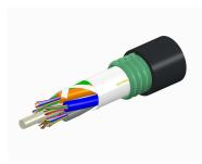
Fiber OSP cable, TeraSPEED® Single Jacket/Single Armor, Gel-Free, 48 fibers, Stranded Loose Tube, Singlemode G.652.D and G.657.A1, Feet jacket marking, Black jacket color
