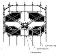
PIM Optimized Adjustable 4-Sector Monopole Platform with 15ft Face - 2-7/8in OD Face Pipes & Top Rail - Includes (20) 2-7/8in OD x 120in Antenna Pipes
