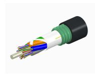
Fiber OSP cable, LightScope ZWP® Single Jacket/Single Armor, 144 fiber, Gel-Free, Stranded Loose Tube, Singlemode G.652.D and G.657.A1, Feet jacket marking, Black jacket color
