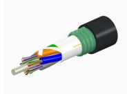
Fiber OSP cable, LightScope ZWP® Single Jacket/Single Armor, 96 fiber, Gel-Free, Stranded Loose Tube, Singlemode G.652.D and G.657.A1, Feet jacket marking, Black jacket color
