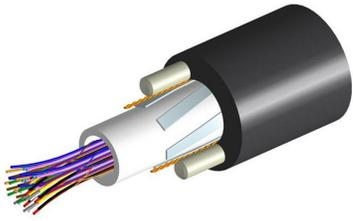
Fiber OSP cable, LazrSPEED® Single Jacket All-Dielectric, Gel-Filled, Central Tube, 48 fibers, Multimode OM3, Feet jacket marking, Black jacket color
