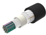
Fiber indoor/outdoor cable, All-Dielectric, LSZH, Riser-Rated, Gel-Free, Central Tube Rollable Ribbon, 864 fiber, Singlemode G.657.A2/B2, Feet jacket marking, Black jacket color, Cca flame rating
