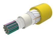
Fiber indoor cable, All-Dielectric, LSZH/Riser-Rated, Gel-Free, Central Tube 200µm Rollable Ribbon, 432 fiber, Singlemode G.657.A2/B2, Feet jacket marking, Yellow jacket color, Cca flame rating
