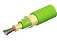
Fiber indoor cable, LazrSPEED® Low Smoke Zero Halogen Riser MPO Trunk Cable, 24 fiber with 24-fiber, 3.0mm subunits, Gel-free, Multimode OM5, Feet jacket marking, Lime green jacket color, B2ca flame rating
