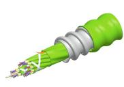
Fiber indoor cable, Plenum MPO Trunk, interlocking aluminum armored with plenum jacket, 144 fiber multi-unit with 16 fiber subunits, Gel-free, OM5 multi-mode, Feet jacket marking, Lime green jacket color
