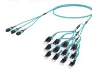
Ultra Low Loss ULL OM4 MPO8 UPC non-pinned to LC/UPC Uniboot Ruggedized fanout Cable, 24-Fiber, Dual Rated (OFNR/LSZH), 8 fiber PmP 2.0 mm
