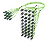
Ultra Low Loss ULL OM5 MPO8 APC non-pinned to LC/UPC Uniboot Ruggedized fanout Cable, 72-Fiber, Plenum, 8 fiber PmP 2.0 mm
