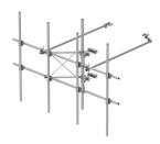
G23RHDX Tower Sector Frame with spine extension for RRU Mounting, 12.5 ft x 2.88 in OD face pipes, includes four 2.88 OD x 120 in antenna pipes
