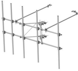
G22HDX High Capacity Sector Frame with 2 7/8in OD x 14.5ft face. Includes five 2 7/8in OD x 120in antenna pipes.
