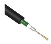
Fiber Optic Outside Plant Cable, 12-core, ECSS (Electro Chrome Coated Steel) Armored, Loose-tube, Gel-filled, 9/125 µm, OS2, Singlemode, Black cable jacket
