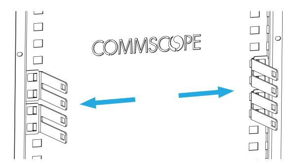
**Step 1:** Prepare the rack with the brackets on the position where you want to install the FACT Chassis (by sliding them in).
