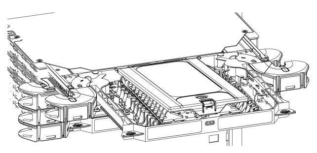
**Step 1:** To remove the cover, rotate the cover about 10° upwards.
