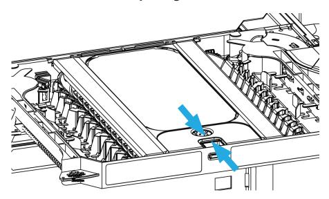
**Step 1:** Apply some force (pinching together in the direction of the arrows) to unlock the cover. Rotate the cover upwards to open it.
