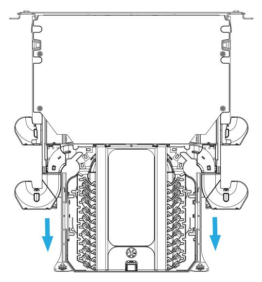
Step 1: Open the upper drawer (releasable). This one is marked at the front (blue marking at the bend control).
