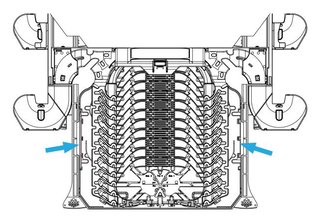
The fiber picker is located on the left or right (as indicated by the arrows). To remove it, simply pull it upwards until it releases from the snapping features.
