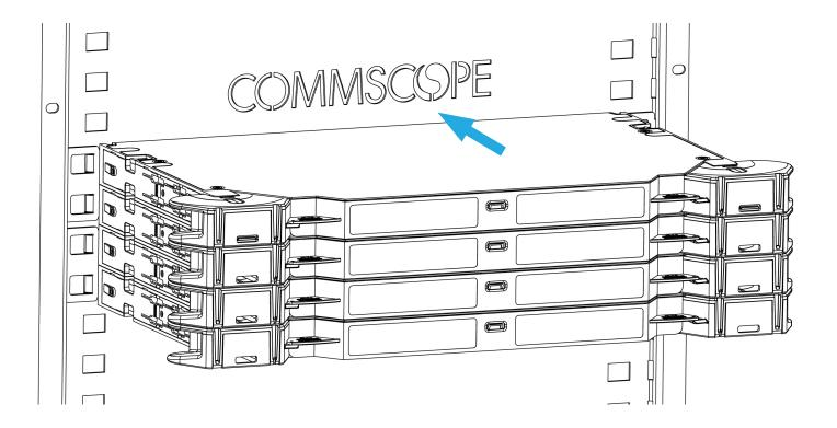
**Step 3:** Slide the FACT Chassis into the brackets until you hear a "clicking noise"..
