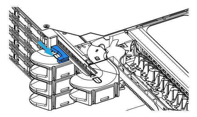
Step 2: Pull the blue puller locks (make sure both sides are in the unlocked position).
