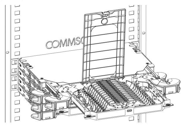
**Step 2:** The cover will stay in the open position if this is rotated about 85°.
