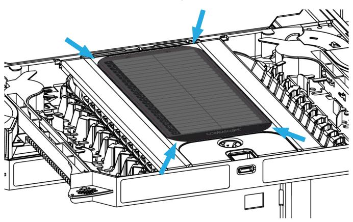
Notes can be made on the label when the cover is closed (this acts as a support). The label can also be removed if preferred. It is held in place in the four corners. Simply slide it out of the four corners to remove.
