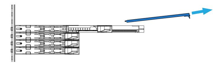
**Step 2:** Pull the cover in the 10° angle towards the front. The cover will pop out of the hinge. To re-assemble the cover, repeat the 2 previous steps the other way around.
