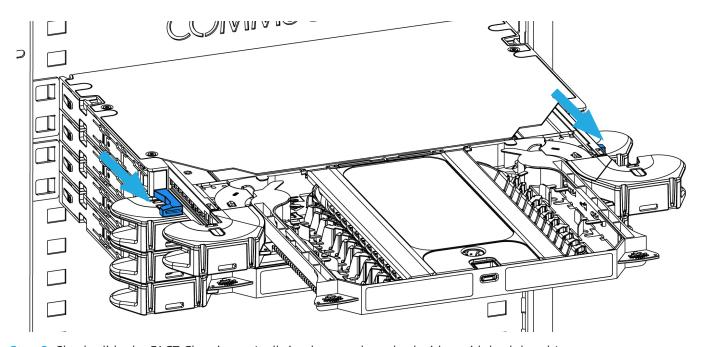
Step 3: Slowly slide the FACT Chassis out (pull simultaneously on both sides, with both hands).
