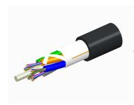
Fiber indoor/outdoor cable, LightSCOPE ZWP® Single Jacket All-Dielectric, LSZH, 24 fiber, Gel-Free, Stranded Loose Tube, Singlemode G. 652.D and G.657.Al, Meters jacket marking, Black jacket color, Eca flame rating
