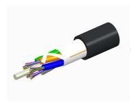
Fiber indoor/outdoor cable, LightSCOPE ZWP® Single Jacket All-Dielectric, LSZH, 48 fiber, Gel-Free, Stranded Loose Tube, Singlemode G. 652.D and G.657.Al, Meters jacket marking, Black jacket color, Eca flame rating
