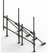
High Capacity DUAL Penetrating Roof Frame, 14 ft face, four 2-7/8 in OD  $\times$  126 in pipes
