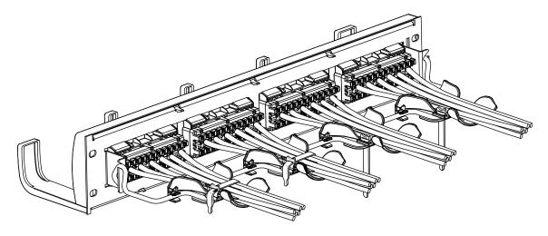
Step 4 - Install Front Cord Management, Front Bezel, Labels and Label Covers
