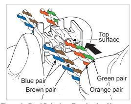
Figure 2. Feed Pairs into Termination Manager
