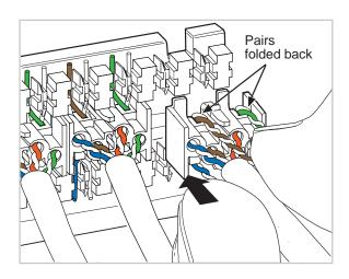
Figure 4. Snap Termination Manager onto Rear Housing
