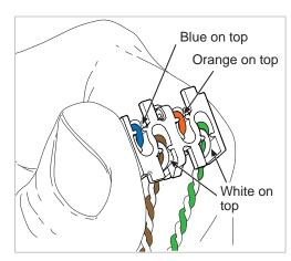
Figure 3. Fold Pairs Back into Slots
