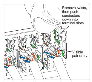
Figure 5. Seat Untwisted Pairs into IDC
