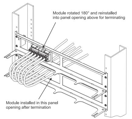
**Module Termination in Multiple Panel Mounting**
