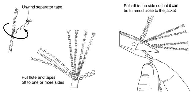
Preparation of the SYSTIMAX GigaSPEED X10D 91B series cable, 95B series cordage, or Xpress<sup>®</sup> 88 series cable is shown above. For complete instructions on preparing the GigaSPEED X10D 91B series cable, 95B series cordage, or Xpress<sup>®</sup> 88 series cable for termination, see instruction sheet 860469402.
