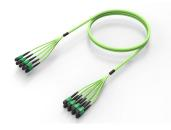
Ultra Low Loss (ULL) OM5 MPO16 APC (Pinned) to MPO16 APC (Pinned), Fiber Trunk Cable Assembly, 128-Fiber, LSZH B2ca
