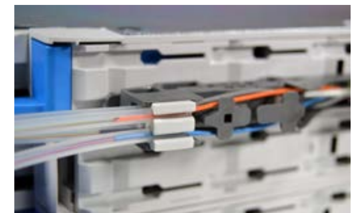
7.1.6. Slide the transportation tube into the tube holder. Make sure that the transportation tube is pushed in, until the end.
