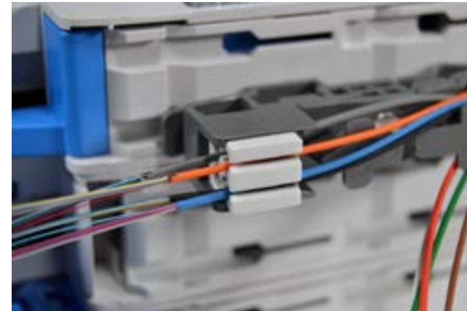
6.1.4. Slide and click the tube holder into the CTU bracket.
