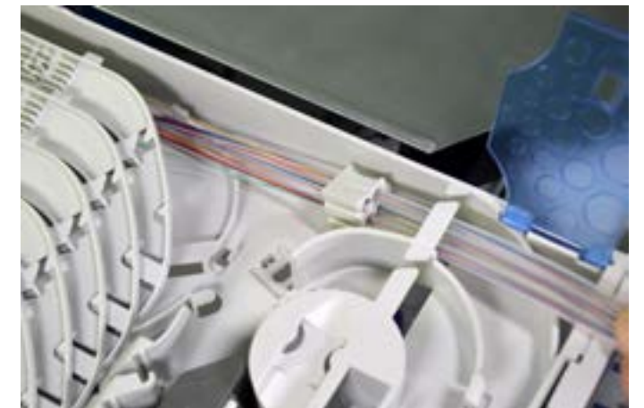
6.1.8. Slide the other sides of the transportation tubes in the another tube holder. Open the lids. Push / slide all transportation tubes one by one into the tray.
