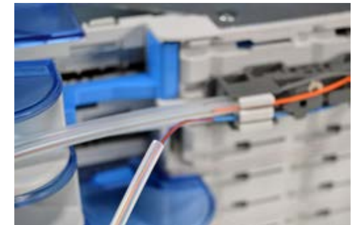
7.1.5. Feed the fibers into the -correct length- transportation tubes.
