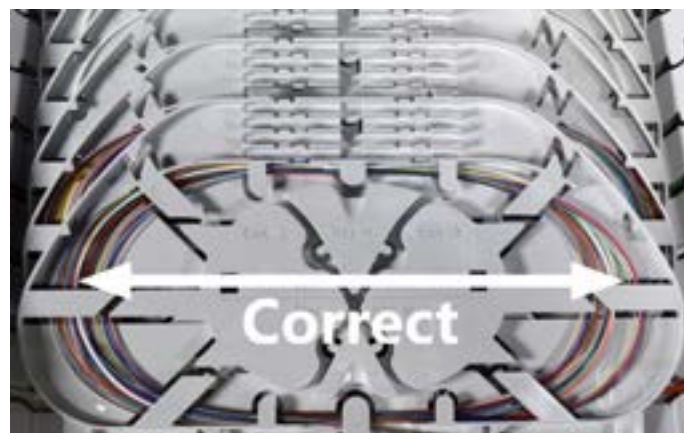
6.12. Pay attention to store the fiber correctly. A properly stored fiber doesn't touch the bend radius limiter on inner or outer side and can move freely.
