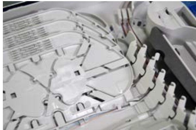
6.2.2. Route the fiber throughout the groove plate to the dedicated splice trays.
