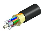
Fiber indoor/outdoor cable LazrSPEED® Indoor/Outdoor Plenum Distribution, 8 fiber single-unit, Multimode OM3, Gel-free, Feet jacket marking, Black jacket color
