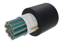
Fiber indoor/outdoor cable, All-Dielectric, LSZH, Gel-Free, Riser Rated, Central Core Rollable Ribbon, 2880 fiber, Singlemode G.657.A2, Feet jacket marking, Black jacket color, Cca flame rating
