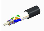
Fiber indoor/outdoor cable, LazrSPEED®, Single Jacket All-Dielectric, Low Smoke Zero Halogen (LSZH), 48 fiber, Gel-Free, Stranded Loose Tube, Multimode OM3, Black jacket color, Feet cable marking, Eca flame rating
