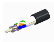
Fiber indoor/outdoor cable, LazrSPEED®, Single Jacket All-Dielectric, Low Smoke Zero Halogen (LSZH), 60 fiber, Gel-Free, Stranded Loose Tube, Multimode OM3, Black jacket color, Meters cable marking, Eca flame rating
