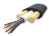
Fiber outdoor drop cable, LightScope® ZWP Self-Supporting All-Dielectric, Singlemode G.652.D and G.657.Al, 12 fiber Arid Core construction, Gel-filled, central loose tube, no ripcords, Meters jacket marking, Black jacket color
