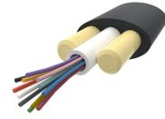
Fiber outdoor drop cable, LightScope® ZWP Self-Supporting All-Dielectric, Singlemode G.652.D and G.657.Al, 12 fiber Arid Core construction, Gel-filled, central loose tube, no ripcords, Meters jacket marking, Black jacket color
