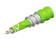
LazrSPEED® Plenum MPO Trunk Cable, interlocking aluminum armored with plenum jacket, 144 fiber multi-unit with 12 fiber subunits
