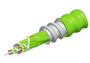
LazrSPEED® Plenum MPO Trunk Cable, interlocking aluminum armored with plenum jacket, 72 fiber multi-unit with 12 fiber subunits
