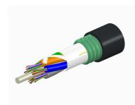
Fiber indoor/outdoor cable, TeraSPEED®, Single Jacket/Single Armor, Low Smoke Zero Halogen (LSZH), Singlemode G.652.D and G.657.A1, 24 fiber, Gel-Free, Stranded Loose Tube, Meters jacket marking, Black jacket color
