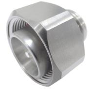
Product Classification Wireless and radiating connector Product Type **Product Brand HELIAX®** General Specifications **Body Style** Straight **Cable Family** LSF2-50 Inner Contact Attachment Method Solder **Inner Contact Plating** Silver Interface 4.3-10 Male **Outer Contact Attachment Method** Solder **Outer Contact Plating** Trimetal Dimensions Length 20.07 mm | 0.79 in Diameter 23.88 mm | 0.94 in
