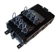
Mini-OTE 300-Series, Optical Terminal Enclosure, 8-port mini-size (DLX®) connector, with integrated 1x8 splitter, black, with grounding, external mounting. Splitter outputs connected to terminal housing ports, maximum 26 splices.
