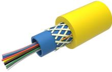
Fiber indoor/outdoor cable, LightScope® ZWP, dry loose tube, 6 fiber, Singlemode G.652.D and G.657.A1, Gel-free, Yellow jacket color, Dca flame rating
