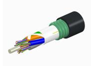
Fiber indoor/outdoor cable, TeraSPEED®, Single Jacket/Single Armor, Low Smoke Zero Halogen (LSZH), Singlemode G.652.D and G.657.A1, 36 fiber, Gel-Free, Stranded Loose Tube, Meters jacket marking, Black jacket color
