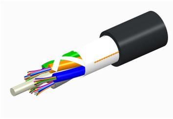
Fiber indoor/outdoor cable, LightScope® ZWP, Single Jacket All-Dielectric, Low Smoke Zero Halogen (LSZH), Singlemode G.652.D and G.657.A1, 12 fiber, Gel-Free, Stranded Loose Tube, Feet jacket marking, Black jacket color, B2ca flame rating
