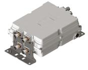
Dual Band Tower Mounted Amplifier, 1800//2100 MHz, 12 dB, 2 BTS & 4 ANT ports, with 4.3-10 connectors, AISG with 1 RET connectors (2 devices with 2 sub-units each)
