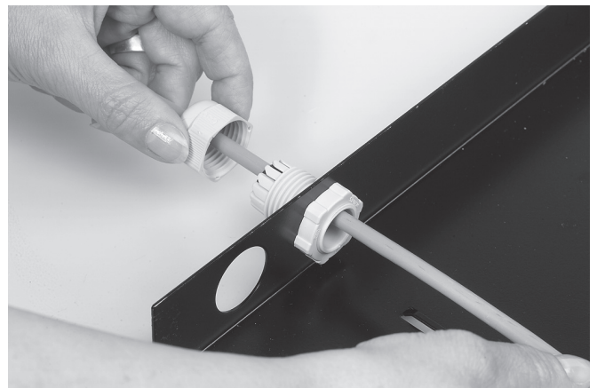
3.2 Push the cable through the gland inside the shelf. Cable entry is provided at both sides on the back of the panel
