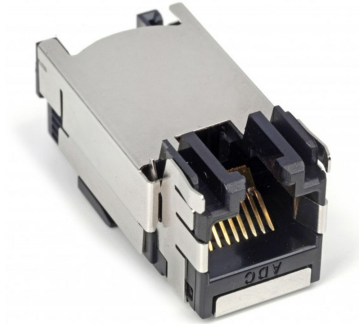
RJ45 Modular Jack Q-Series, category 6A, shielded, 8-position
