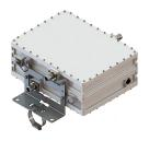
Tri Band Tower Mounted Amplifier, 1800/2100/2600 MHz, 12 dB, 2 BTS & 2 ANT ports, AISG with 1 RET connector (3 devices with 2 sub-units each), with 4.3-10 connectors
