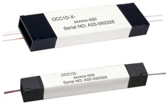
OCC1D DWDM, 1 channel, double demux, 1535.82 nm starting wavelength, 0.250 mm cable, light duty housing, field installable
