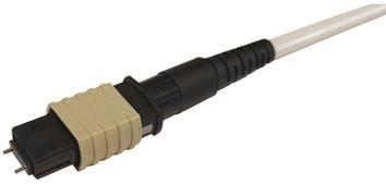
Qwik-Fuse MPO Connector, PINNED, OM1, Beige, for 3.0 mm round cable, two per pack
