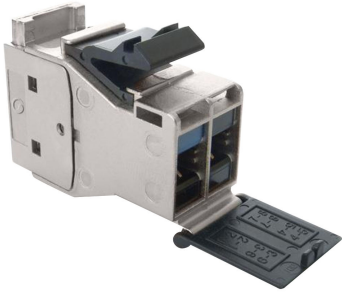
AMP-TWIST SL-Series Modular Jack, 8-position, category 7AS, shielded, with dust cover
